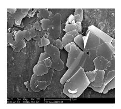
Hexagonal boron nitride (h-BN) is the equivalent in structure of graphite. Like graphite its plate like microstructure and layered lattice structure give it good lubricating properties. Sinyo supply three series powder, like LN, HW and SA for different purpose. For example, LN series, we can supply 2-4microns or 4-7microns, also 8-12microns powder for your selections.
